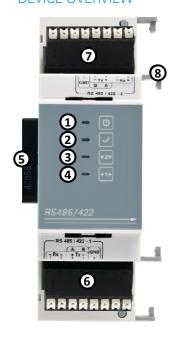
LED: Power Status (1) 2 LED: Device Status LED: Bus-2 Connection 3 4 LED: Bus-1 Connection (5) Connector for blue'Log expansion 6 Interface for RS485/422 - 1 7 Interface for RS485/422 - 2 8 Case lock
