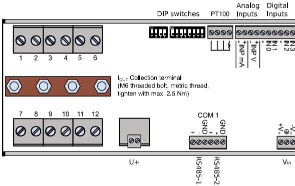
Fig. 2: Device overview – front side of the String Monitoring Unit 1225
