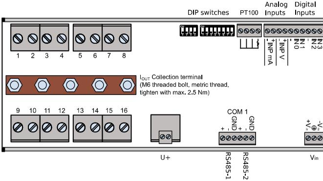
Fig. 3: Device overview – front side of the String Monitoring Unit 1625
