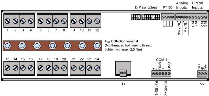
Fig. 4: Device overview – front side of the String Monitoring Unit 2422
