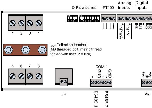
Fig. 1: Device overview – front side of the String Monitoring Unit 0825
