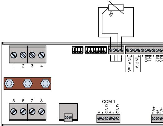
Fig. 6: Connecting a PT100 temperature sensor
