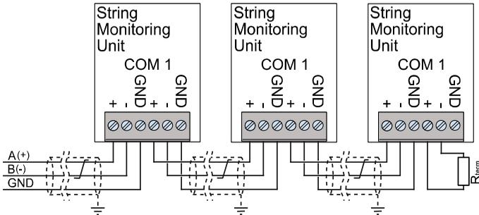
*Fig. 7: Daisy-chain cabling*
