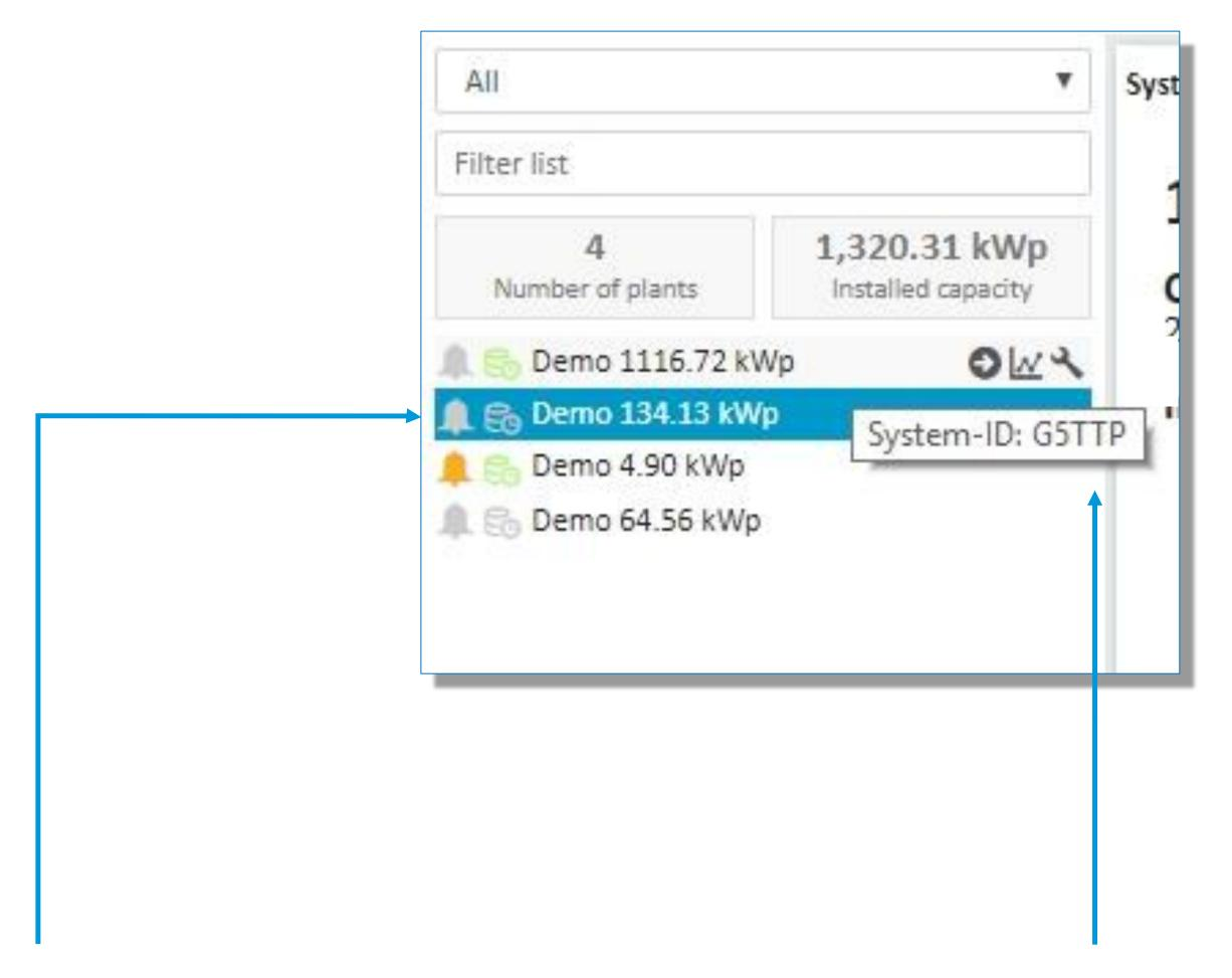
SYSTEM INDICATORS – The bell icon indicates open alarms, and the database icon indicates data input problems. Ideally, both should be green. If the icons are gray, this means that alarms are in progress or that there is no available data input.
