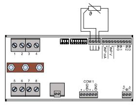
Fig. 6: Connecting a PT100 temperature sensor
