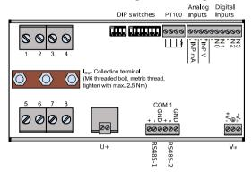
Fig. 1: Device overview – front side of the String Monitoring Unit 0825
