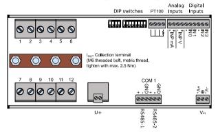
Fig. 2: Device overview – front side of the String Monitoring Unit 1225
