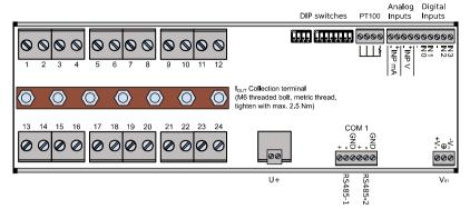
Fig. 4: Device overview - front side of the String Monitoring Unit 2422
