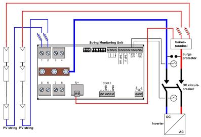
Fig. 5: Typical circuitry for a String Monitoring Unit
