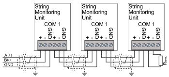
Fig. 7: Daisy-chain cabling
